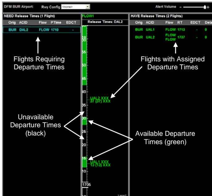
Figure 4. Prototype DFM ATCT Interface
