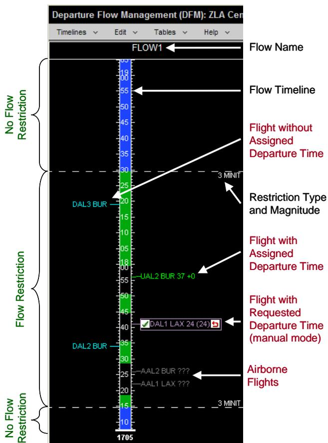
Figure 3. Single Flow Timeline on Prototype DFM ARTCC Interface
