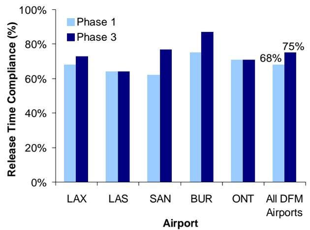
Figure 7. ZLA Departure Release Time Compliance, Showing Overall Increase When DFM is Used
