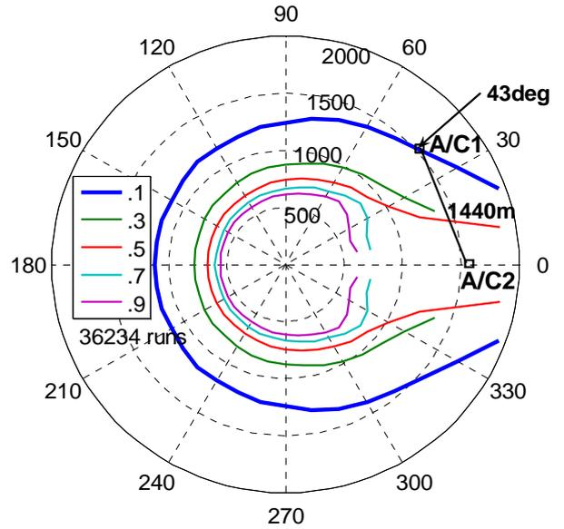
Figure VI. Iso-lines of constant collision probability around the path intersection
