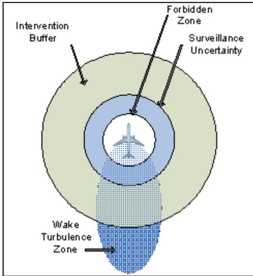
Figure III. Common separation component breakdown
