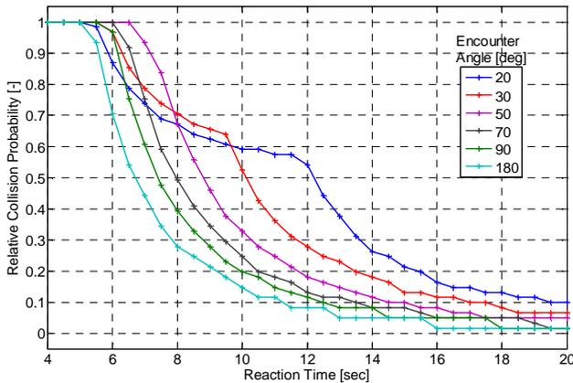
Figure V. Collision probability vs. reaction time (seconds before collision), both a/c at a speed of 100m/sec, 25m forbidden zone radius
