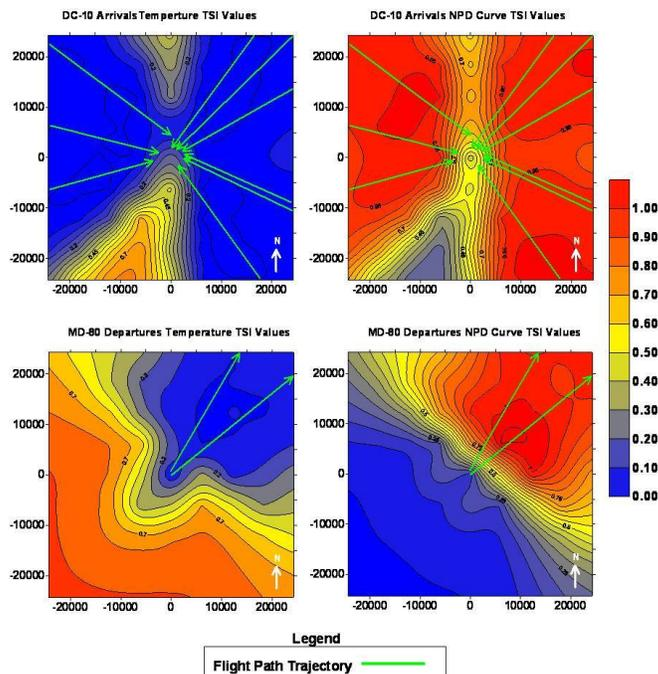
Figure 4: AAM GSA results for the temperature and NPD curve inputs for DC-10 arrivals and MD-80 departures
