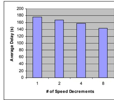
**Figure 5. Effects of Path and Speed Discretization on Arrival Delay**
