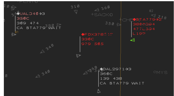
Example: High climb rate of BTA779 causes 3 near-term conflicts (TSAFE issues left turn)
