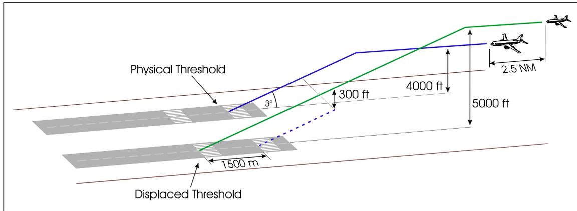
Figure 1. Displaced threshold approaches on a dependent runway system
